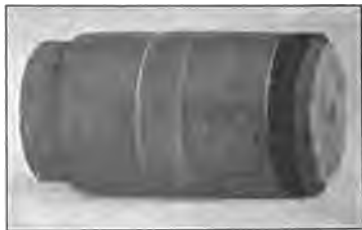
Fig. 150. Mallet with Iron Rings.
